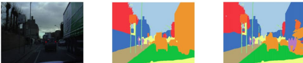
Figure 2.6: From Left original image, original annotation (ground truth) masks and predicted masks
