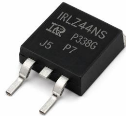
Figure III.17: MOSFET Power Switch(IRLZ44NS)
