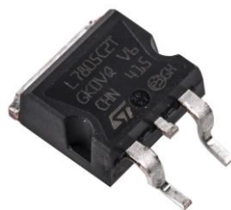
Figure III.10: L7805CD2T Voltage Regulator Circuit.
