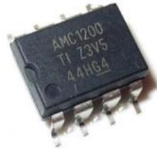
Figure III.23: current Measurement (AMC1200)
