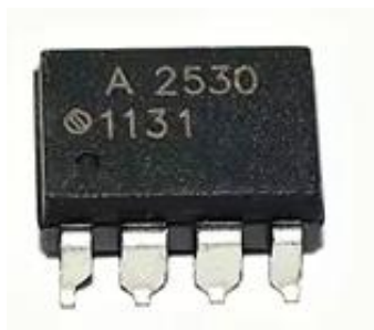
Figure III.6: HCPL-2530 Optocoupler Circuit.
