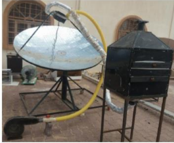
Fig. I.20: Solar Parabolic Dish Concentrator (PDC) for drying [38].
