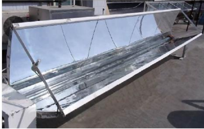
Fig. I.18: Air heating using a multi-surface trough solar concentrator [36].
