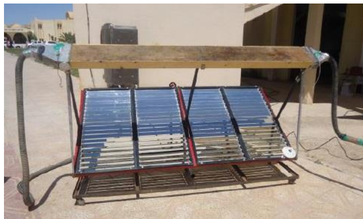
Fig. I.17: Linear Fresnel Reflector (SAHLFR) solar air heater with a rectangular duct absorber [35].
