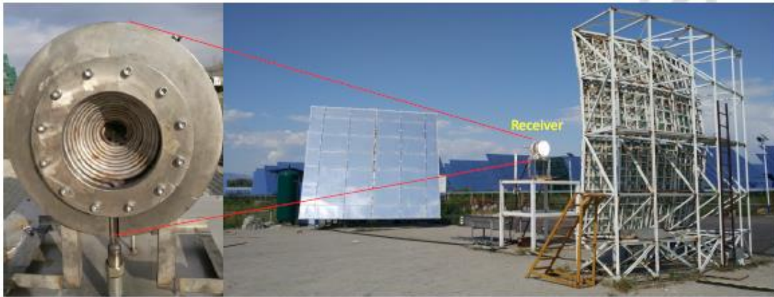
Fig. I.19: Tubular air receiver in solar dish system [37].
