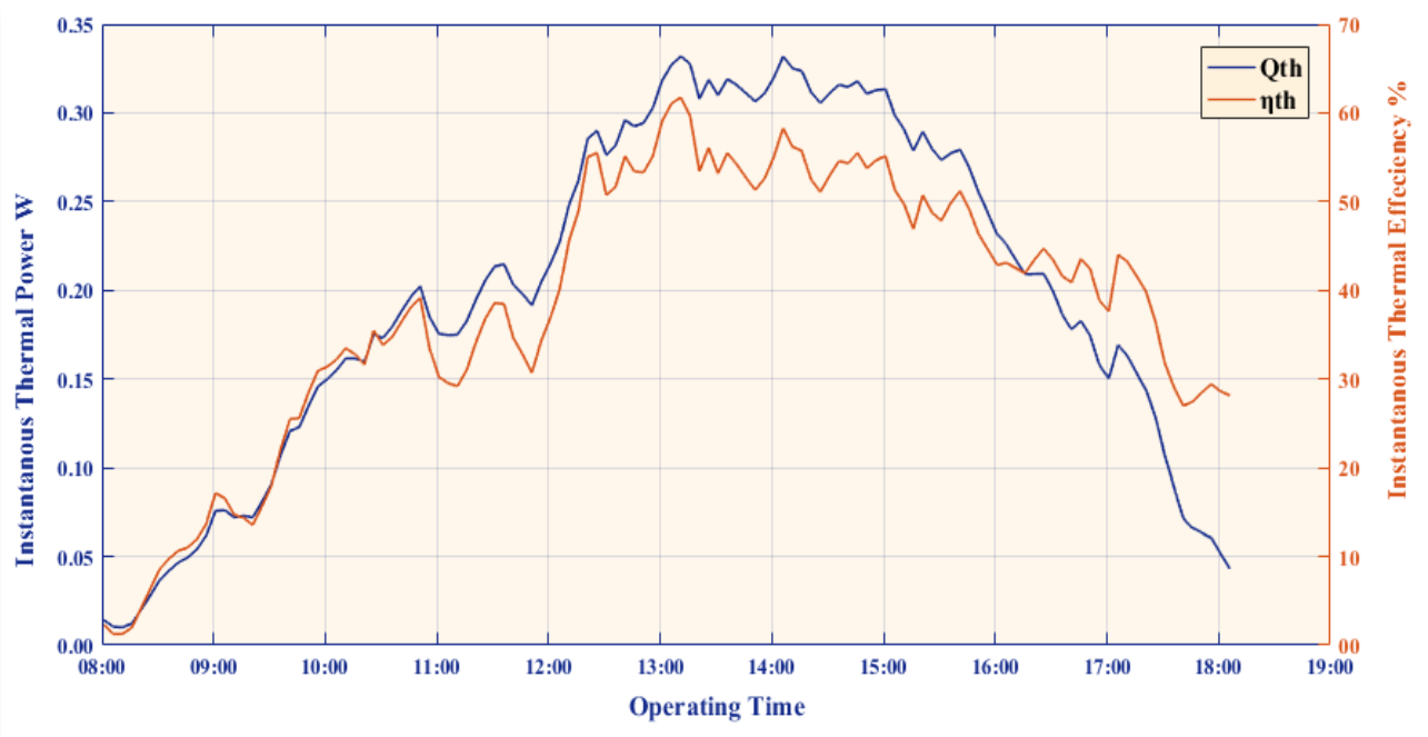
Fig. 4-5: Instantaneous Thermal Output and Efficiency Variation.
