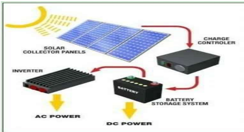
Figure I.10 requires a voltage regulator in anticipation of keeping the battery from damage.
