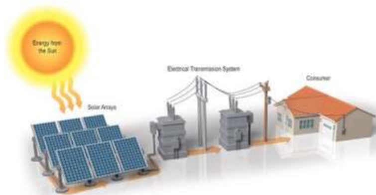
Figure (I.9): Solar power generation
