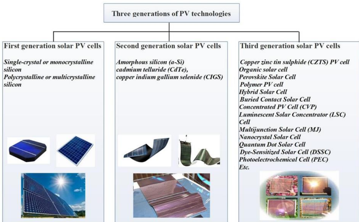
Figure I.11: The three generations of solar photovoltaic (PV) cells. [6]
