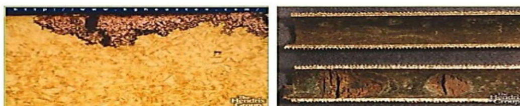
Figure I.5: Selective corrosion of brass (Cu-Zn) [29]
