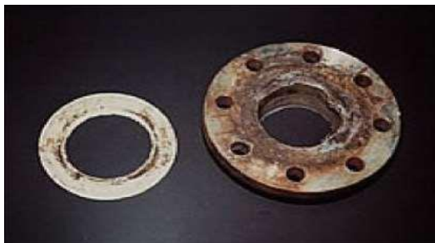
Figure I.6: Cavernous corrosion of an alloyed steel under a joint [30].
