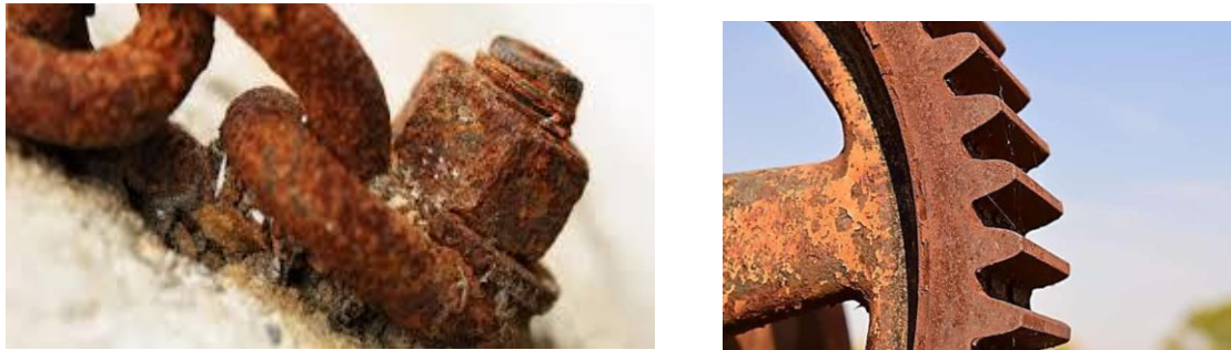
Figure .I.1: Pictures of materials subjected to corrosion phenomena
