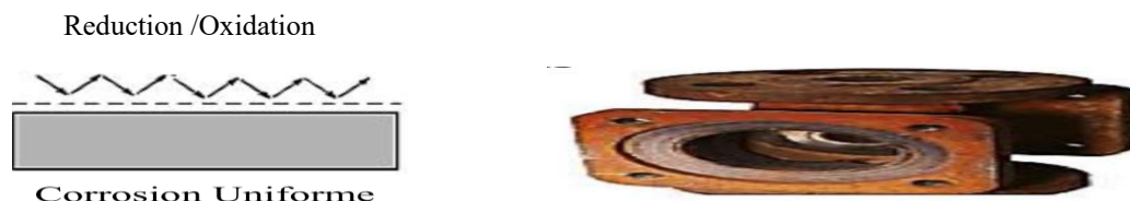
Figure I.2: General corrosion (rust) of a piece of steel [22,23]
