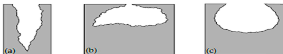
Figure I.4: Types of punctures (a) deep cavity (b) cavernous cavity (c) hemispherical [29]
