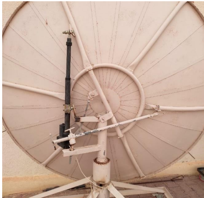
Figure II. 5: Photo of the tracking system containing a cylinder and a rotary axis.
