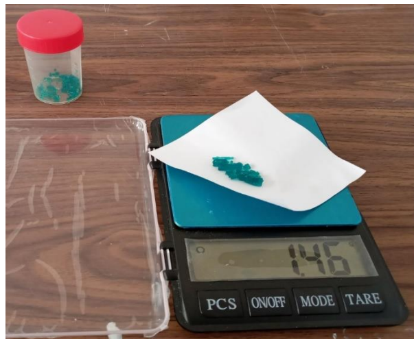
Figure II. 13: Sensitive electrical balance MH-999.
