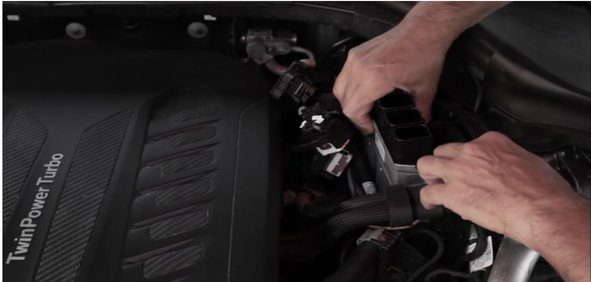
Figure 57: ECU connecting with engine connection
