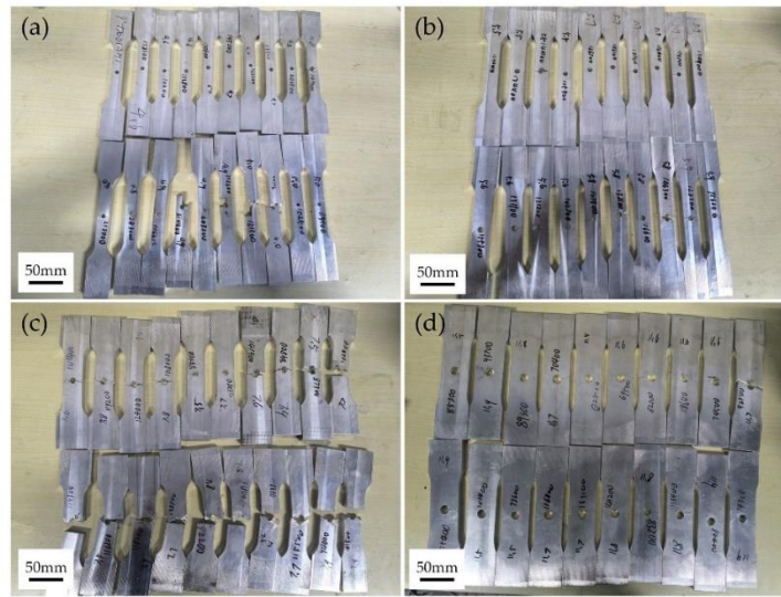
Figure II.9 Cold expansion specimens with different initial hole diameters after fatigue testing: (a) 4.3 mm; (b) 5.3 mm; (c) 7.18 mm; (d) 11.1 mm
