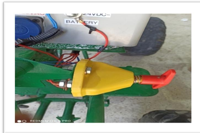
Figure III.18. Circuit coup courant
