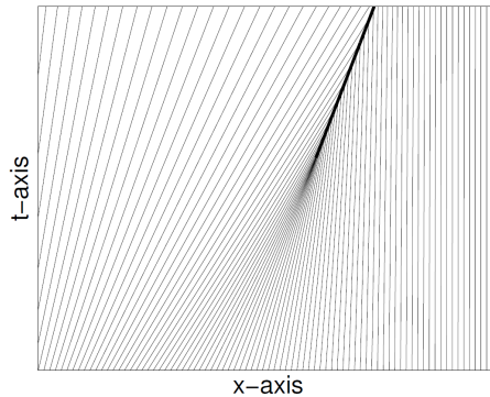
FIGURE 1.2 – A shock wave in Burgers equation for the initial speed given by V(x)=\exp(-x^2) . The heavy black line is where the collisions happens.
