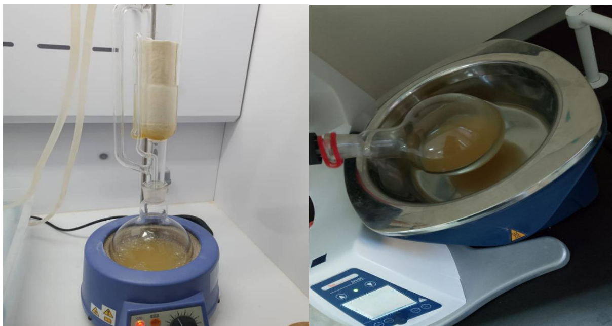
Figure 01: Extraction method of methanol and water mixture.
