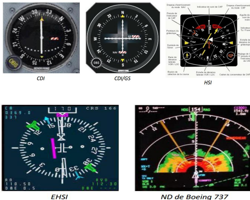
Figure II.12 : Instrument de diverses formes CDI, CDI/GS, HSI, EHSI, ND [21].
