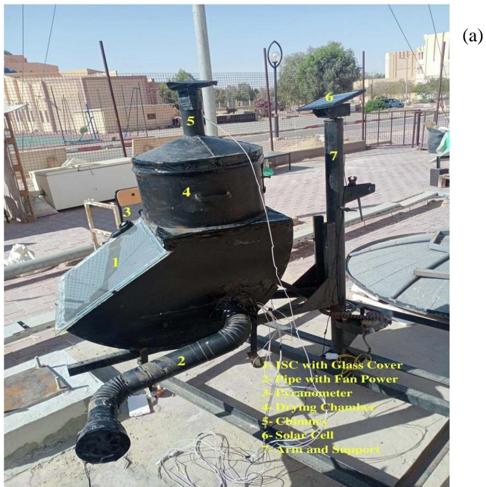
Figure (0-7): Reversed absorber type solar dryers
