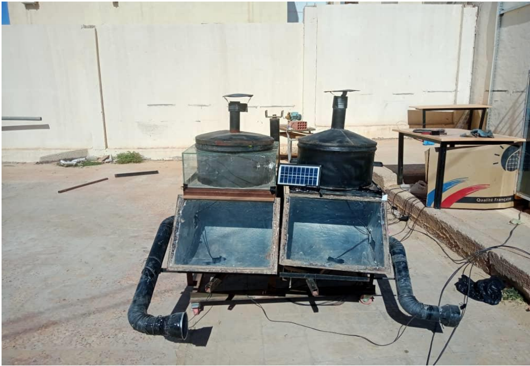
Figure (III-10): A photograph of ISD components in tracking system.
