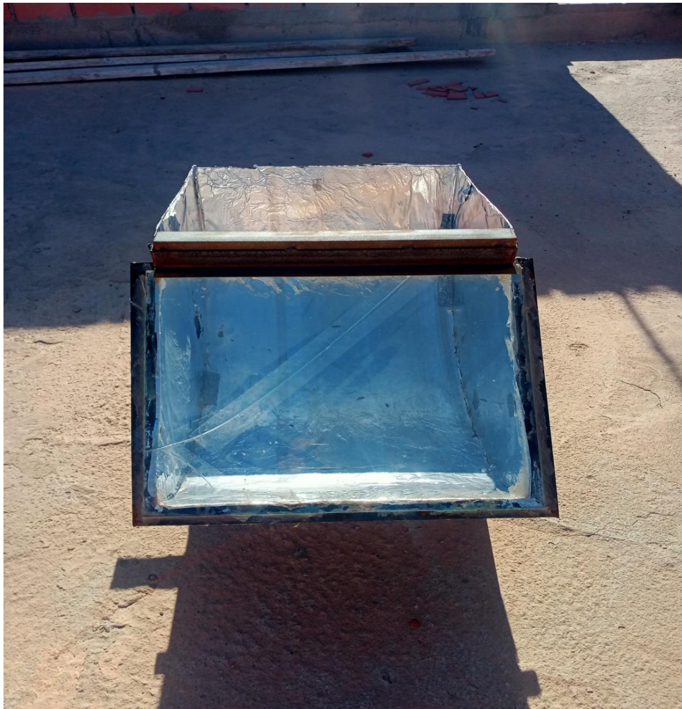
Figure (0-9): Photograph of the inverted solar collector [26].
