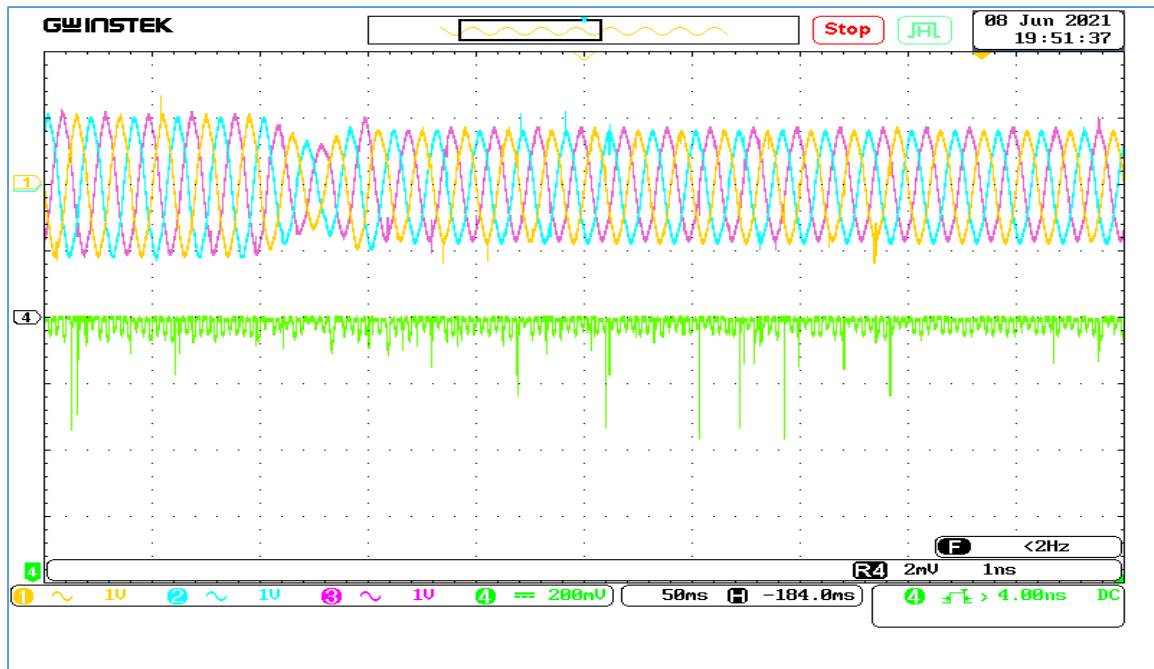
Fig n°44: Three-phase Voltage and Frequency
