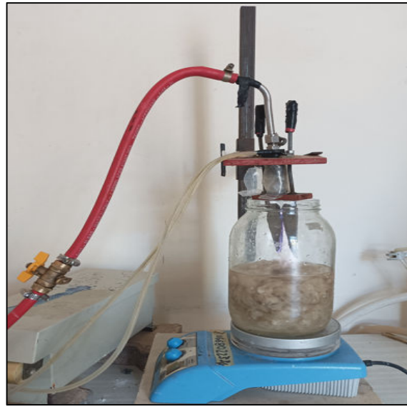
Figure IV.5: Wool fiber under cold plasma jet.
