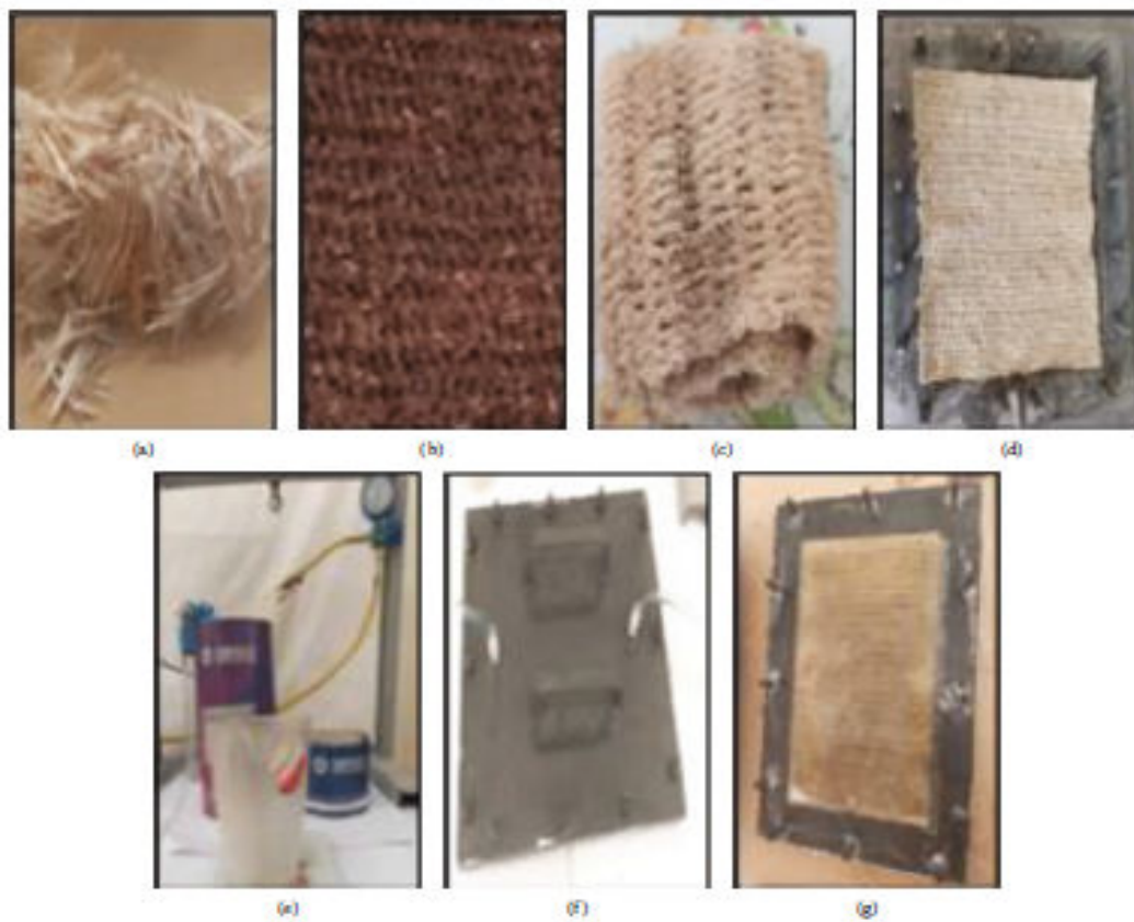
FIGURE 7: Manufacturing of composites by vacuum infusion molding: (a) Periploca laevigata Aitton fiber, (b) WLF, (c) NWLF, (d) PLAF-WIF, (e) epoxy and hardener, (f) closed mold, and (g) composite after curing time.
