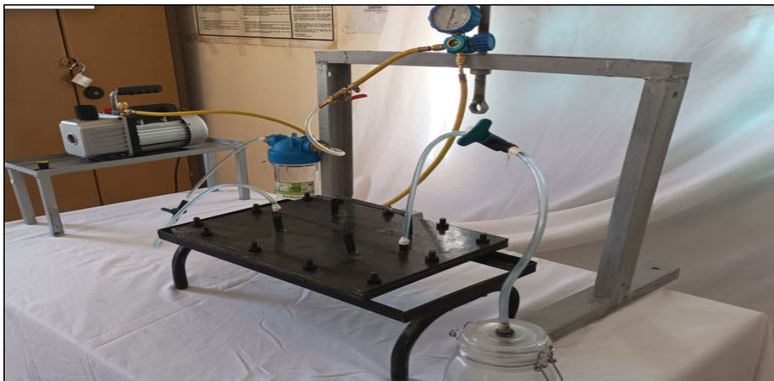
Figure IV.11: Vacuum Infusion Molding Process for Composite Material Manufacturing.
