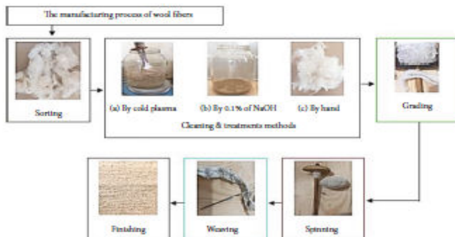
FIGURE 3: Preparation of the wool fiber: (a) cold plasma treatment, (b) treatment by 0.1% NaOH, and (c) manual cleaning.
