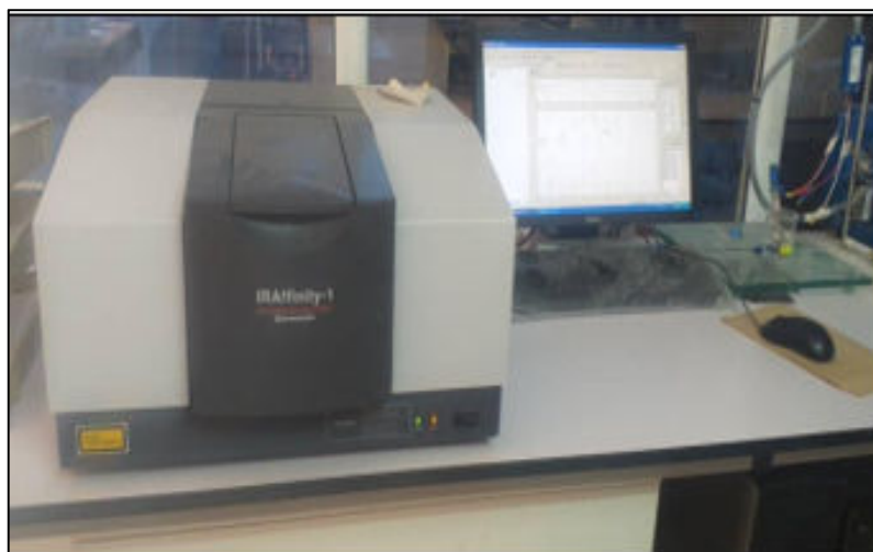
Figure IV.7: Shimadzu, IR Affinity-1, Fourier Transform Infrared.
