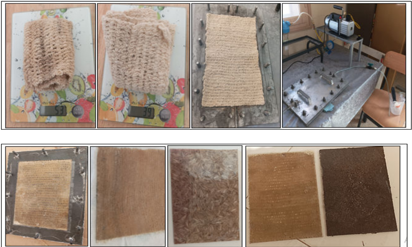
Figures IV.12: Manufacturing process steps, and the final products.
