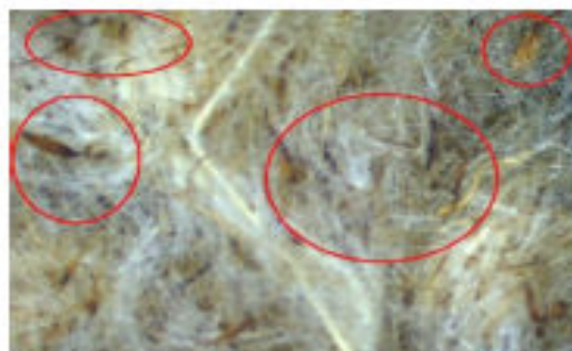
FIGURE 18: Optical microscope image of microscope image of untreated wool fiber indicates the presence of the impurities.
