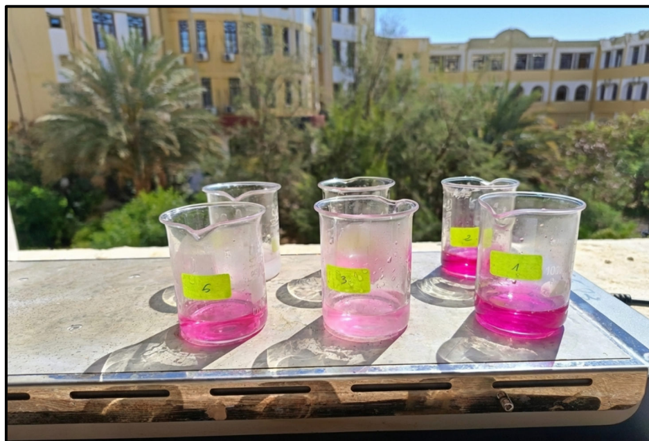
Figure (IV.3): Photodegradation of Rose Bengal under natural solar light irradiation using \text{ZnFe}_2\text{O}_4 nanoparticles.
