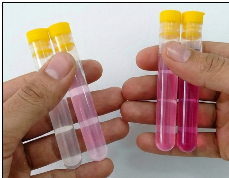
Figure (IV.4) : Photograph showing the visual decoloration of Rose Bengal aqueous solution after photocatalytic degradation using \text{ZnFe}_2\text{O}_4 nanoparticles under natural solar irradiation; the tubes on the right show the initial intense pink-colored dye solution prior to irradiation, while the tubes on the left show the nearly colorless treated solution after 90 minutes of sun exposure.
