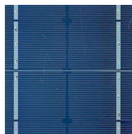
Figure (I. 5) Cellule photovoltaïque monocristalline
