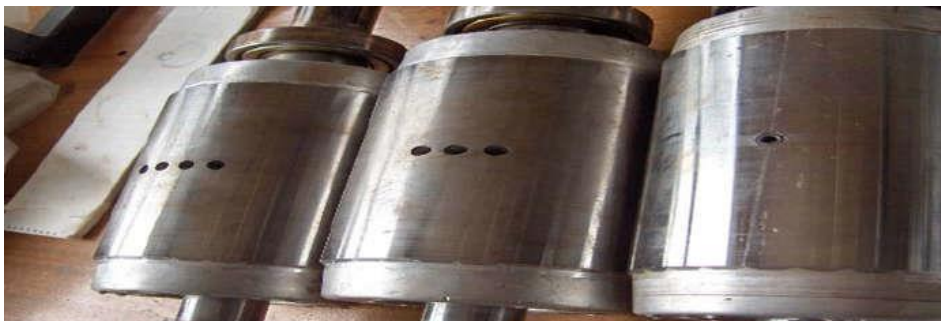
Figure I. 5. Ruptures de barres
