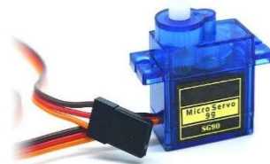
Figure II. 10 : servo motor G90 .
