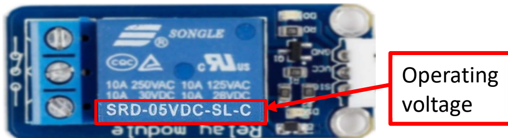
Figure II. 22: Relay operating voltage.
