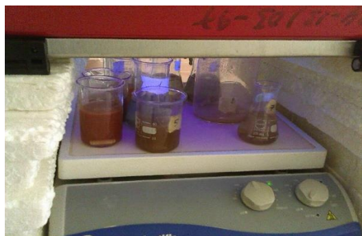
Fig.9. Test of photodegradation ( Vat Green 03 textile dye ) of the mixtures ( \text{TiO}_2 + DB ) and ( \text{TiO}_2 DMF1 ) in the photocatalytic reactor ( transilluminator )
