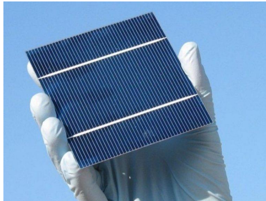
Figure (1.9): photovoltaic cell
