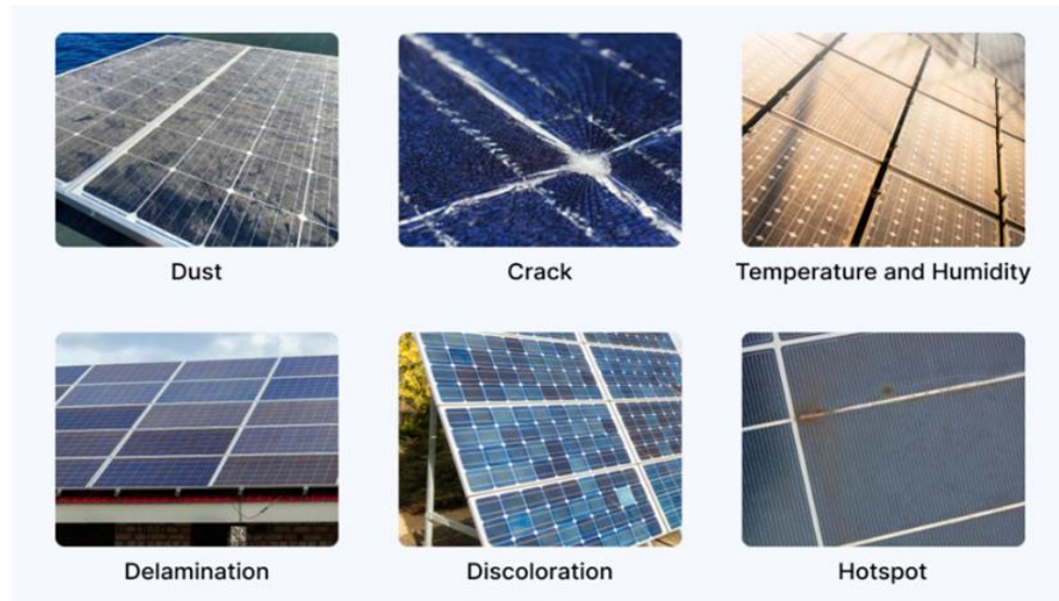
Figure (1.16): Key Factors Leading to Solar Panel Degradation
