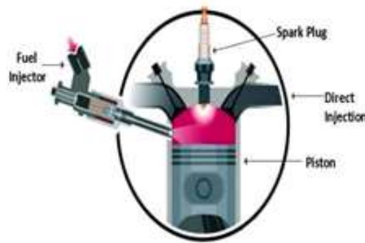
Figure I.28. Injection directe de carburant [14]
