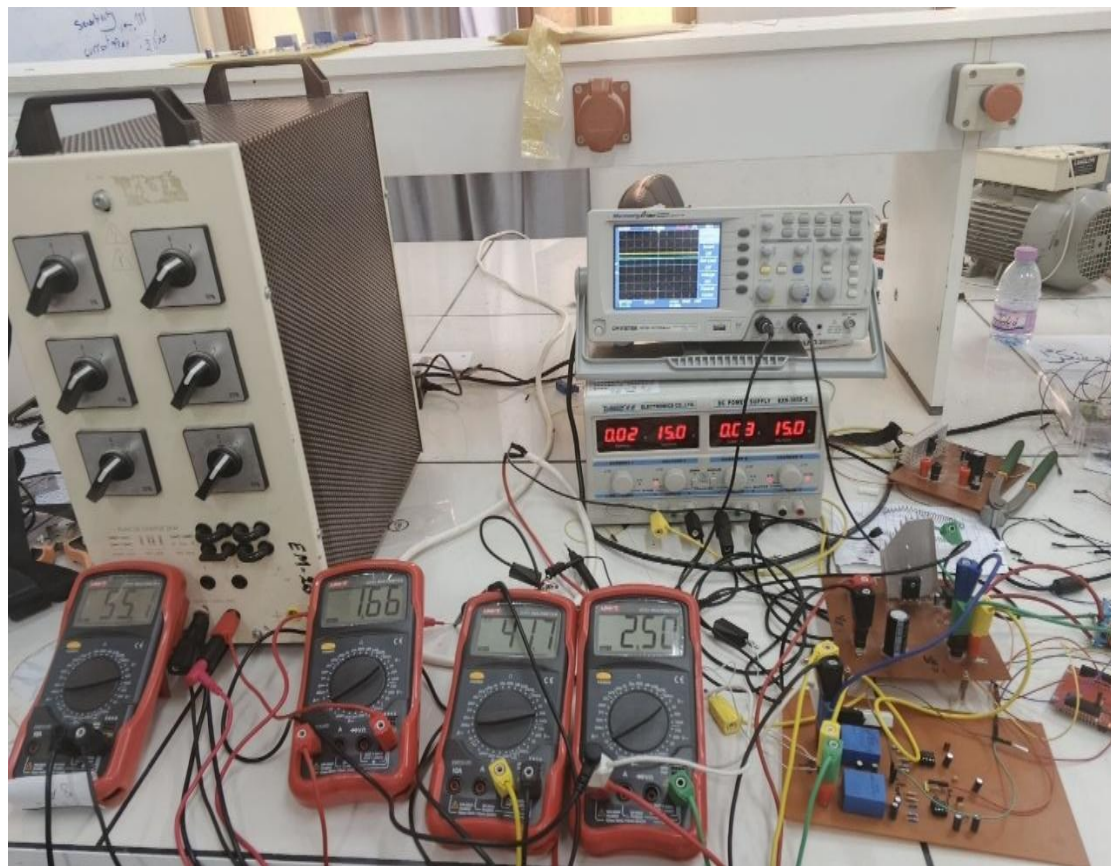
Figure .III.17: Experimental Investigation of the Designed System P&O MPPT Technique in high Irradiance
