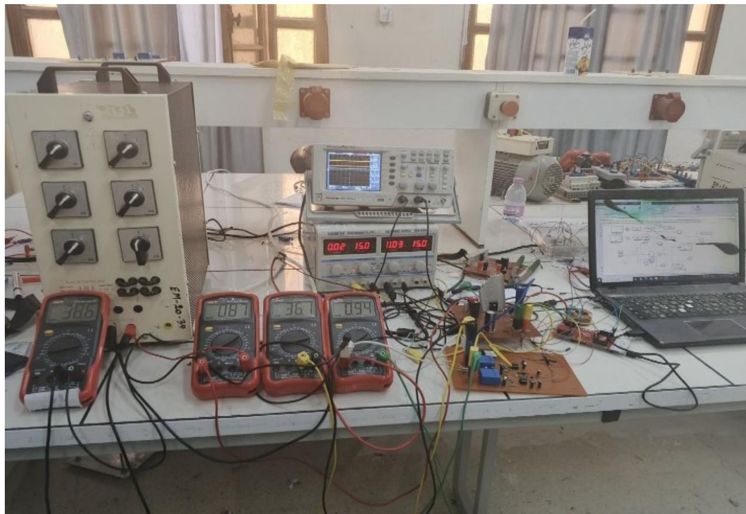
Figure .III.14: Experimental Investigation of the Designed System P&O MPPT Technique in low Irradiance
