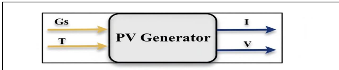
Figure 1.12: Block Diagram of a PV Generator
