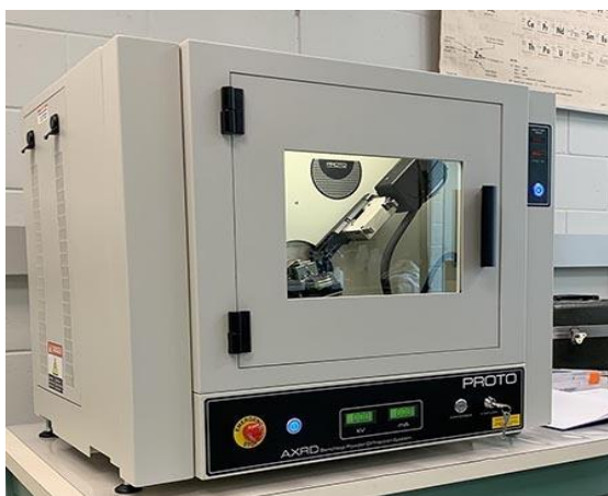
Figure II.5: Benchtop X-ray diffractometer (XRD) apparatus used to determine the crystalline structure, phase purity, and crystallite size of the synthesized nanomaterials.
