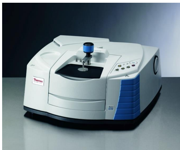
Figure II.7: Fourier-Transform Infrared (FTIR) spectrometer employed for identifying surface functional groups and confirming the presence of plant-derived capping agents.
