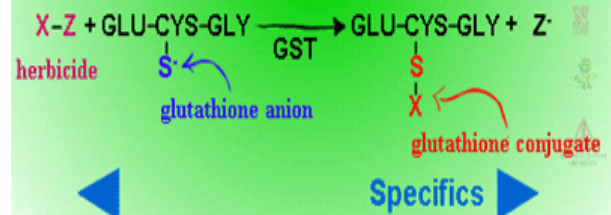
Fig. 20: Glutathione conjugation with herbicides (X) containing halogen, phenolate or alkyl sulfoxide groups (Z)
