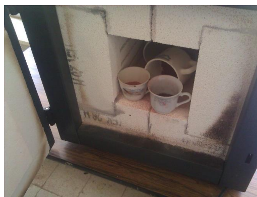
Fig.4. Diatomite silica doped iron nanoparticle with thermally calcination at 600 °C ( DMF3X6) in oven
