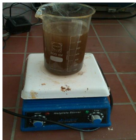
Fig.2. Diatomite silica doped iron nanoparticle with thermally calcination at 600 °C ( DMF3X6) during stirring and heating
