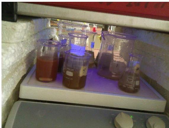
Fig.17. Test of photodegradation ( Vat Green 03 indanthren dye textile ) in presence diatomite silica doped iron nanoparticle thermally calcination at 600 °C “ DMF3X6 ” in the photocatalytic reactor ( transilluminator ) The discoloration efficiency of the catalyst was calculated by the following equation Eq. (4)
