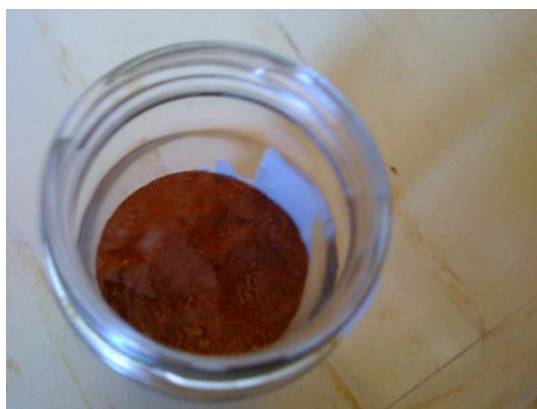
Fig.5. Diatomite silica doped iron nanoparticle with thermal calcination at 600 °C (DMF3X6) in powder
