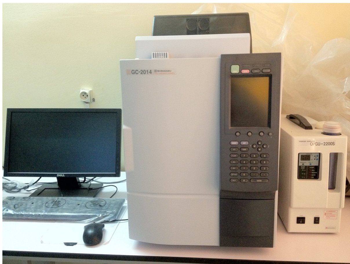
Figure 2.2 A commercial gas chromatograph (Shimadzu GC – 2014 courtesy of the VTRS laboratory) with a flame ionization detector.
