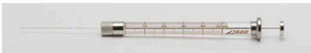
Figure 2.4 Typical syringes used in GC (SGE 5 \mu\text{L} courtesy of VTRS laboratory).
