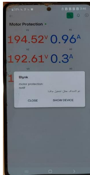
Figure 3.33: Dry running fault alert.
