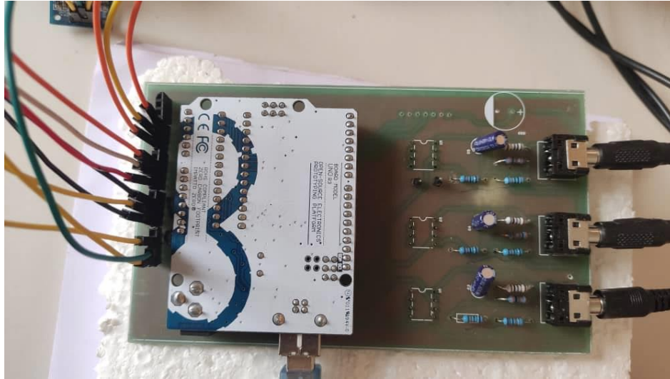
Figure 3.17: Final design and manufacture of printed circuit board.
