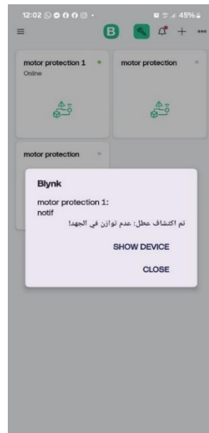
Figure 3.29: Unbalanced fault alert.
