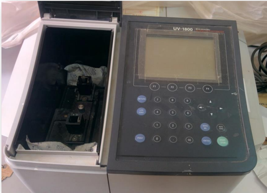
Figure 35: Experimental UV-visible spectroscopy device UV-1800 used
