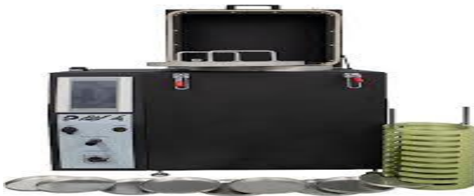
Figure 1.10: L'essai PAV (Pressure Aging Vessel - EN 14769)
