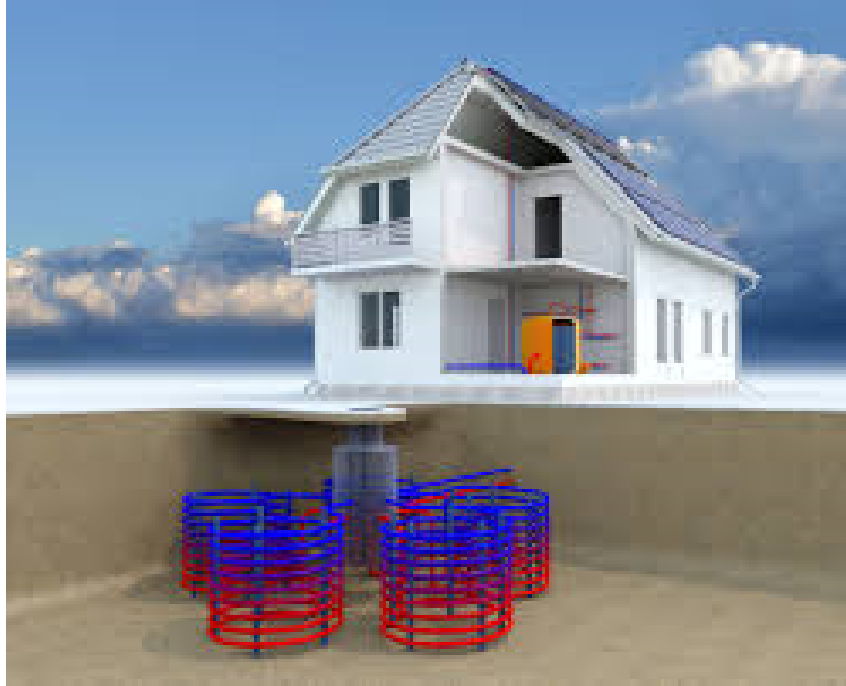
Figure I.15: Schematic representation of helical sensors
