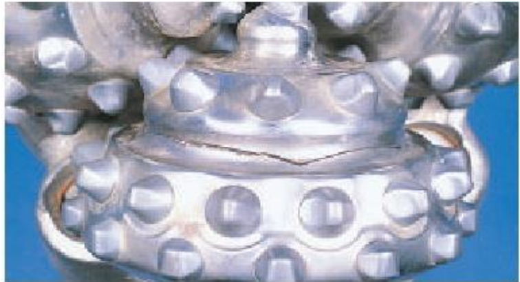
CRACKED CONE (CC)
