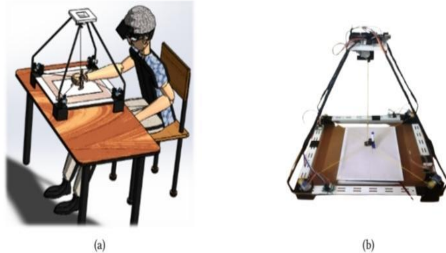
Figure 1.4: Pyramidal cable driven robot: (a) concept; (b) prototype at UNICAL.
