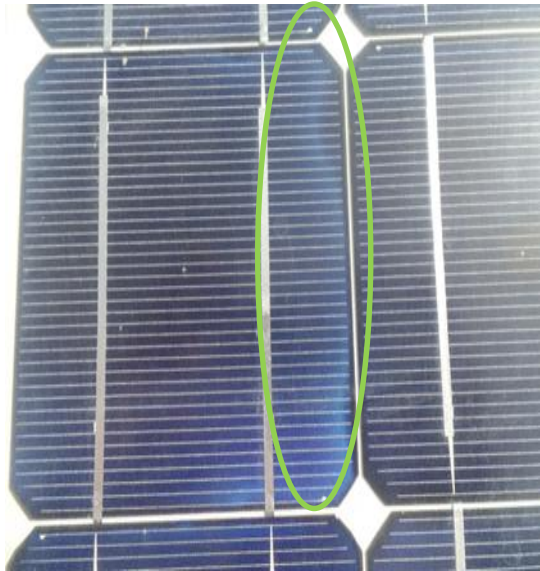
Fig.5. Antireflection coating damage
