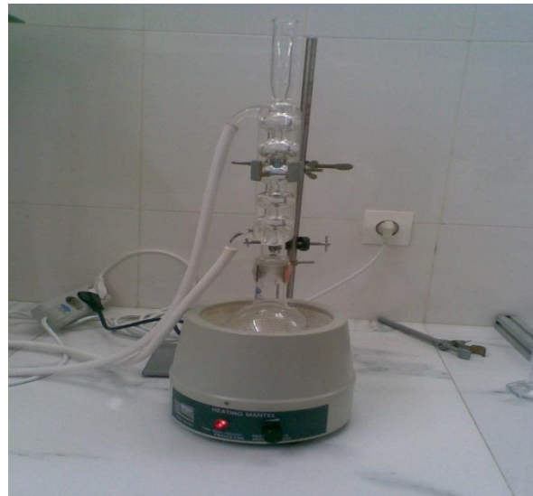
Figure 22: chauffe –de ballon (photo originale).
