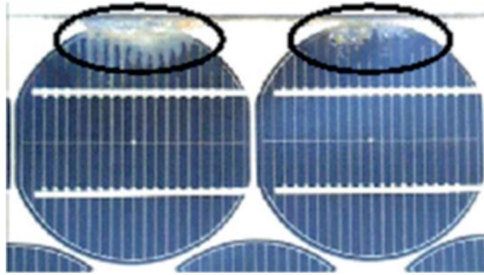
Figure I.20: delamination solar cell module
