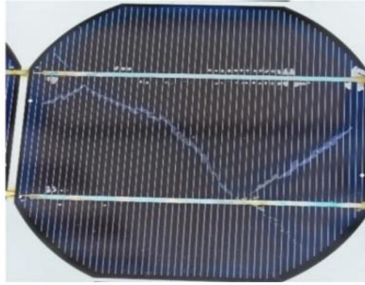
Figure I.19: illustrated the crack of the solar cell.
