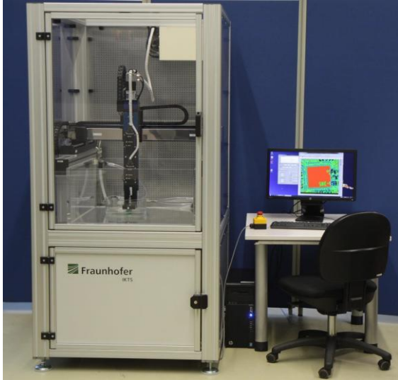
Fig(1): Experimental Device (Variable Ultrasonic Scanner "VariUS")
