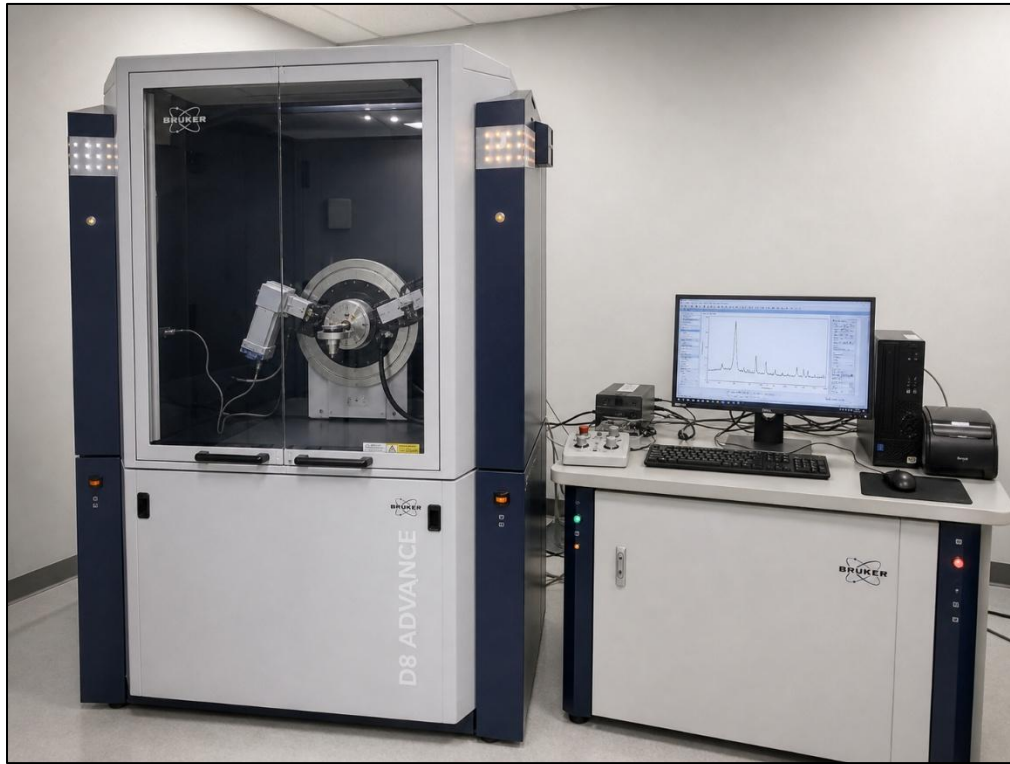
Figure 2. 7 Photo of the Bruker D8 Advance diffractometer used in this work.
