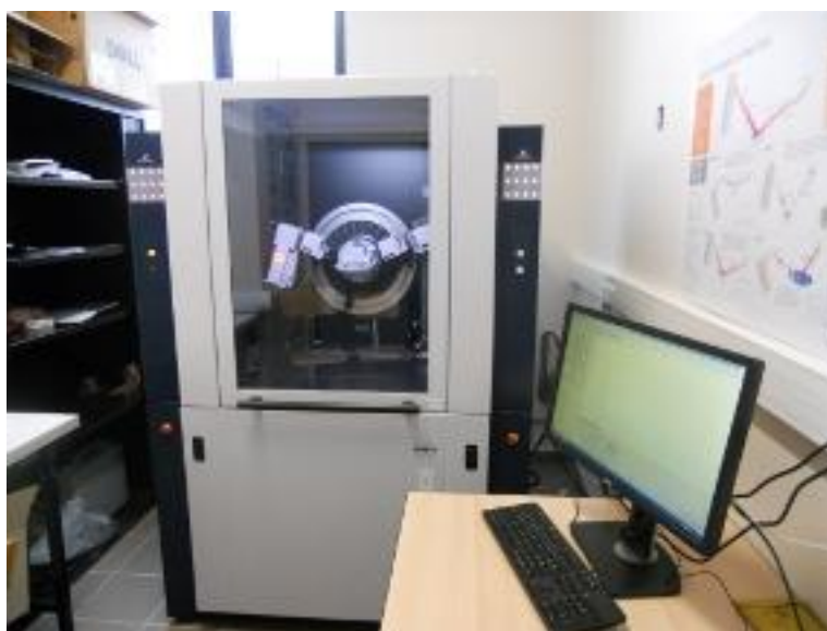
Figure II.6 : diffractomètre de type D8 Advance Bruker
