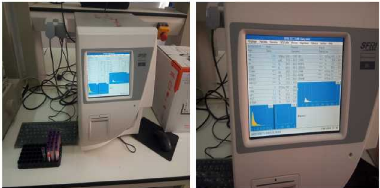
Figure 04: Analyseur hématologique de type SFRI BCC 3 diff (photo originale., 2018).
