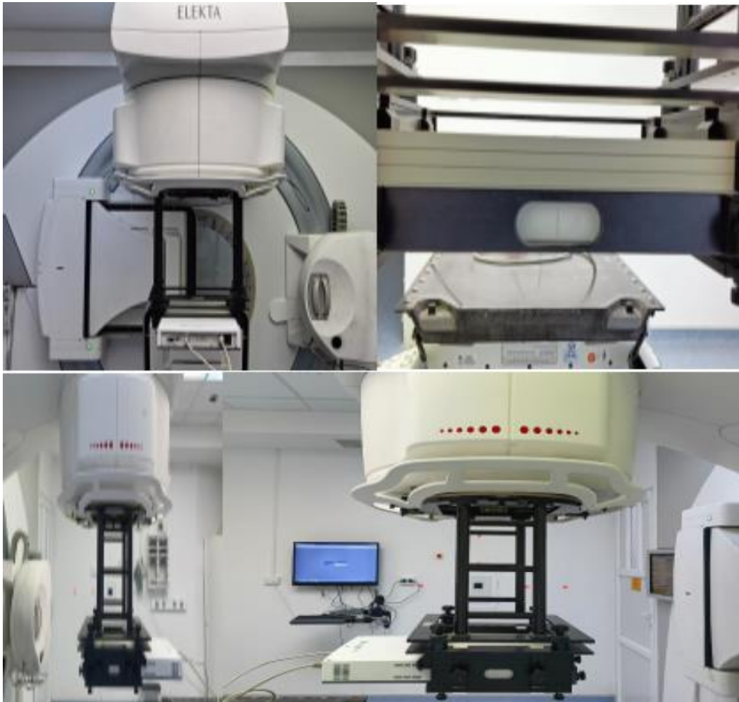
Figure IV.3 : matrices xx + plaque de PMMA
