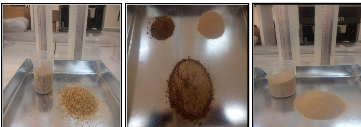
PhotoIII.6: Sable grossier, mélange sable + EC, sable sec.
