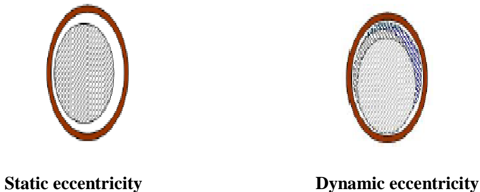
Fig I.9 Schematic modeling of static and dynamic eccentricity [9]
