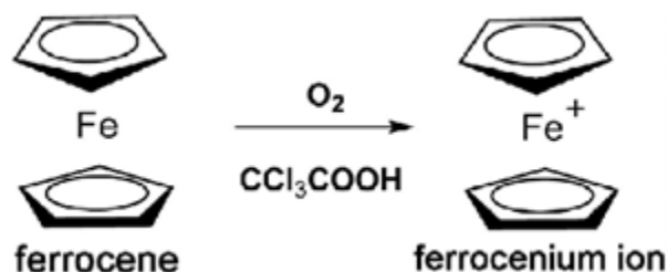
Figure I-15 Oxidation reaction of ferrocene to ferrocenium ion
