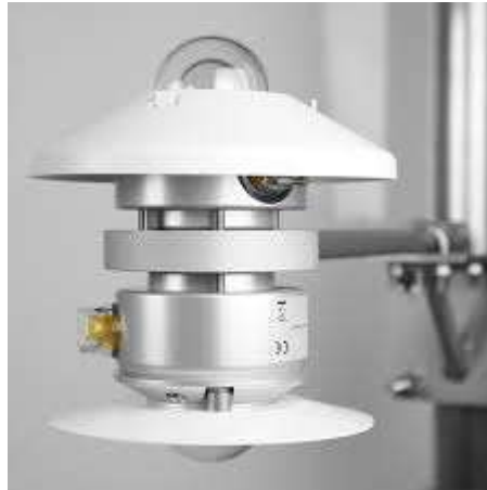
Figure III.5: Albedometer for measuring reflected solar radiation [31].
