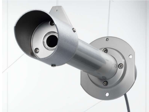
Figure III.3: Pyrhelimeter instrument for direct beam radiation measurement [31].
