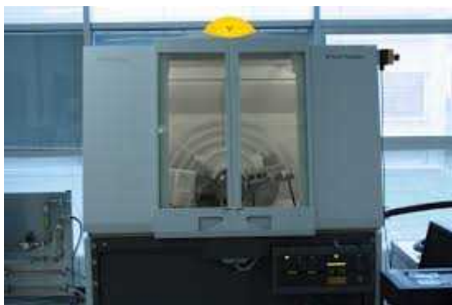
Figure III .2: Diffractomètre vertical, D8 ADVANCE (BRUKER)
