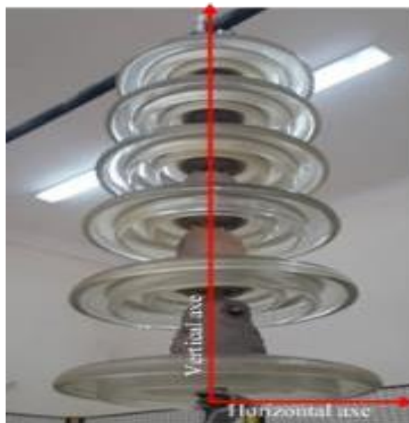
Figure II-10 The Chain of Insulators Used and the Measurement Axes of the Field
